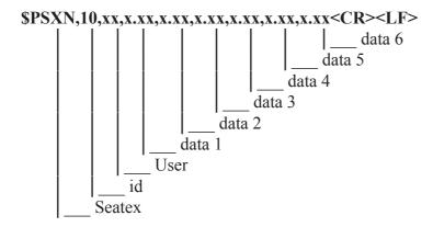
**Note:** For the Seatex protocol to run at an Data Update Frequency of 100Hz the sensor bit rate must be set at a minimum of 57600. To run the sensor at a Bit Rate of 38400 the Data Update Frequency needs to be below 78Hz. Failure to do this may result in problems with the output data.
