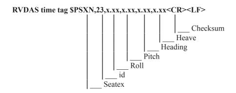
**Note:** For the SEAPATH protocol to run at an Data Update Frequency of 100Hz the sensor bit rate must be set at a minimum of 115200. To run the sensor at a Bit Rate of 57600 the Data Update Frequency needs to be below 81Hz & for 38400 54Hz. Failure to do this may result in problems with the output data.
