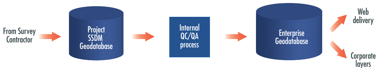
Figure 7: The OGP SSDM workflow from survey contractor to corporate delivery of seabed survey data
