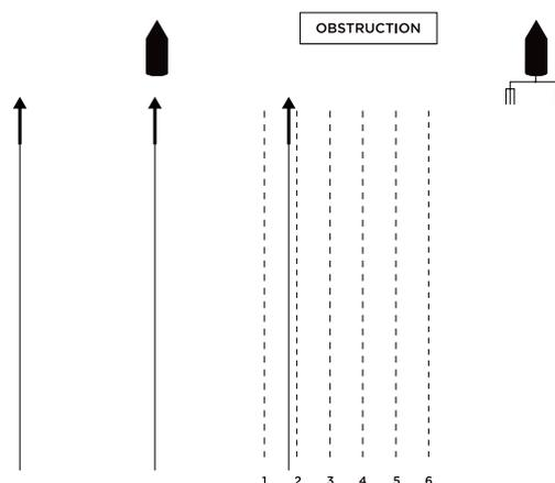
Figure 10 – Triple streamer, dual source undershoot geometry (credit: Chris Walker)
