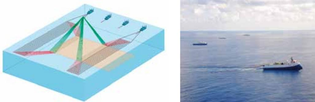
Figure 12 – Wide-azimuth towed streamer geometry (credit: WesternGeco)
