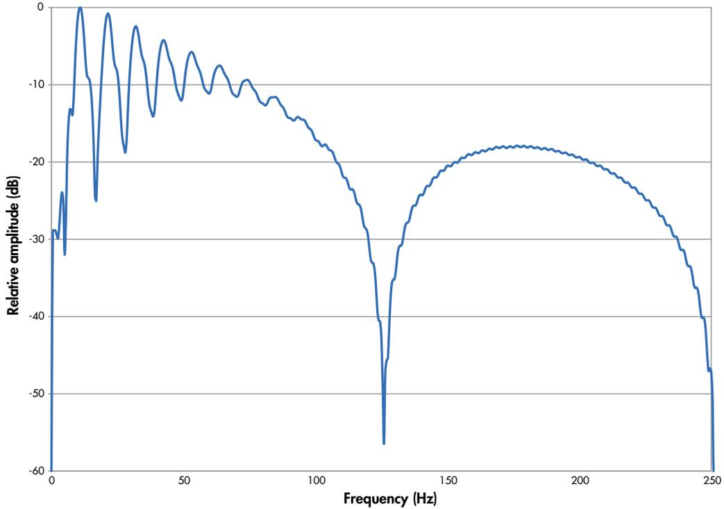
Figure 18b – Amplitude spectrum of a single airgun (credit: Polarcus)
