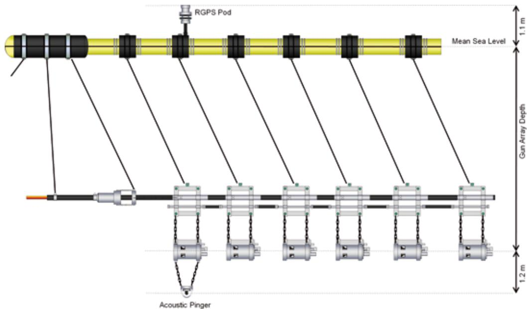
Figure 21a – Side view diagram of a sub-array (credit: Polarcus)
