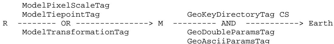
The geocoding coordinate system is defined by the GeoKeyDirectoryTag, while the Georeferencing information (T) is defined by the ModelTiepointTag and the ModelPixelScale, or ModelTransformationTag. Since these two systems are independent of each other, the tags used to store the parameters are separated from each other in the GeoTIFF file to emphasize the orthogonality.
